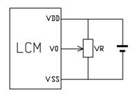
$V_{\text{DD-}}V_0\text{: LCD Driving voltage}$
